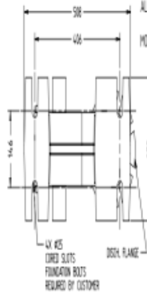
FOOTPRINT OF DISCHARGE ELBOW STAND
